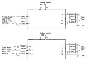
Figure 3-3 Connection diagram of main circuit
