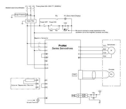
■ Three-phase 400V ProNet-10D~75D/ Three-phase 400V ProNet-E-10D~50D
