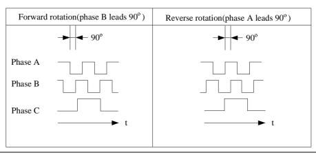
If a servomotor is not equipped with the absolute encoder, servomotor needs two circles rotation before using the serivedr ive's phase-C pulse output for zero point reference.
