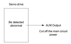
Normally, the external circuit consists of /ALM should be able to switch off power of servo drive.
