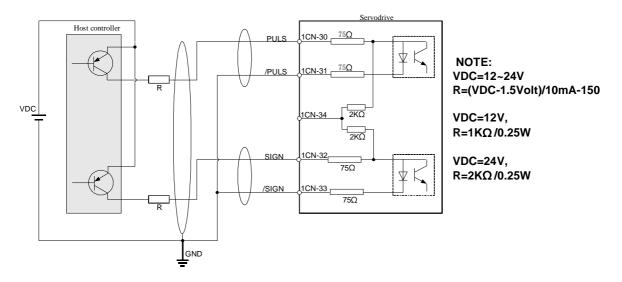
**Note:** When the host controller applied by open-collector signal output, input signal noise margin lowers. When a position error caused by the noise occurs, set the parameter Pn006.3.
