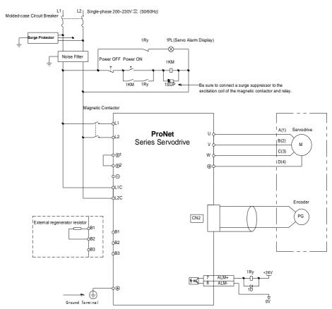
Note 1.The L1,L2,L3 and L1C,L2C terminals wiring method of ProNet-02A~04A/ProNet-E-02A~04A servo drives is different from other ProNet series servo drives. Please note the specific terminal definition while wiring.
