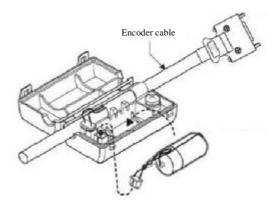
C.Cover the shell of the battery case.
