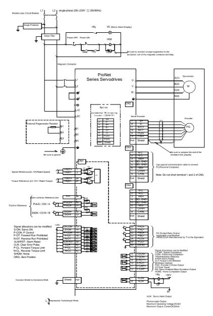
Note 1.The L1,L2,L3 and L1C,L2C terminals wiring method of ProNet-02A~04A/ProNet-E-02A~04A servo drives is different from other ProNet series servo drives. Please note the specific terminal definition while wiring.
