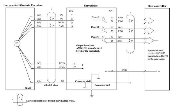
Note: (1)There are no BAT+ and BAT- signals in incremental encoder. (2)The pin numbers for the connector wiring differ depending on the servomotors.
