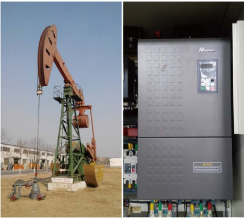
Easydrive inverter applied for beam-pumping unit
