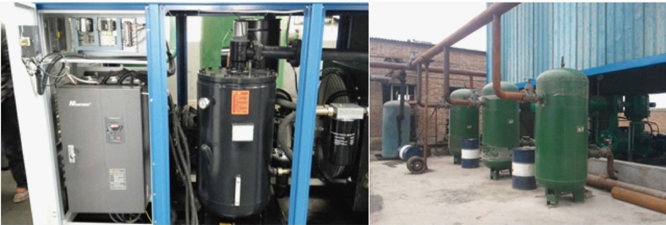
Easydrive 132kw inverter applied for air compressor
