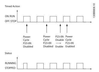
Illustration 3.58 Reactivation Test Diagram
