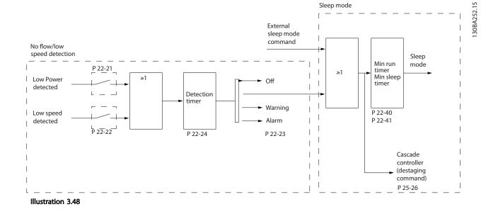
The frequency converter includes functions for detecting if the load conditions in the system allow the motor to be stopped:
