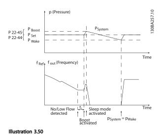
If no flow is detected, the frequency converter will increase the set point for pressure to ensure a slight over pressure in the system (boost to be set in 22-45 Setpoint Boost). The feedback from the pressure transducer is monitored and when this pressure has dropped with a set percentage below the normal set point for pressure (Pset), the motor will ramp up again and pressure will be controlled for
