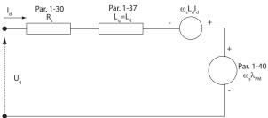
q-axis equivalent circuit
