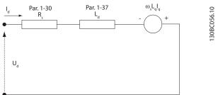
d-axis equivalent circuit
