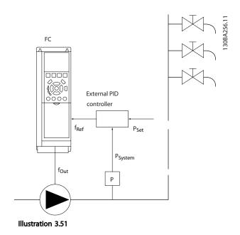
2) In systems where the pressure or temperature is controlled by an external PI controller, the wake up conditions can not be based on feedback from the pressure/temperature transducer as the setpoint is not known. In the example with a boost system, desired
