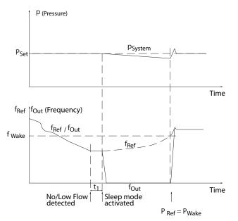
When low power or low speed is detected the motor is stopped, but the reference signal (f<sub>ref</sub>) from the external controller is still monitored and because of the low pressure created, the controller will increase the reference signal to gain pressure. When the reference signal has reached a set value f<sub>wake</sub> the motor restarts.
