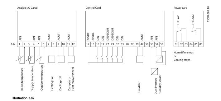
This shows a typical Air Handling Unit (AHU). As can be seen, the addition of the Analog I/O option offers the possibility to control all of the functions from the frequency converter, such as inlet-, return- and exhaust dampers or heating/cooling coils with temperature and pressure measurements being read by the frequency converter.
