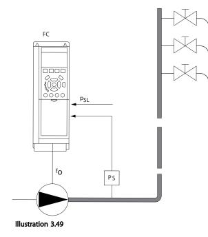
1) Systems where the integrated PI controller is used for controlling pressure or temperature e.g. boost systems with a pressure feed back signal applied to the frequency converter from a pressure transducer. *1-00 Configuration Mode* must be set for Closed Loop and the PI Controller configured for desired reference and feed back signals.
