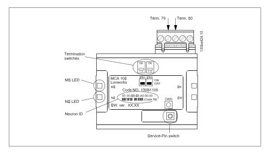
The LonWorks option is equipped with two termination switches, S300 and S301, enabling double termination when using bus topology.
